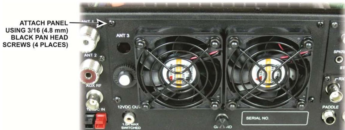
Figure 17. Fan Panel Installed.
