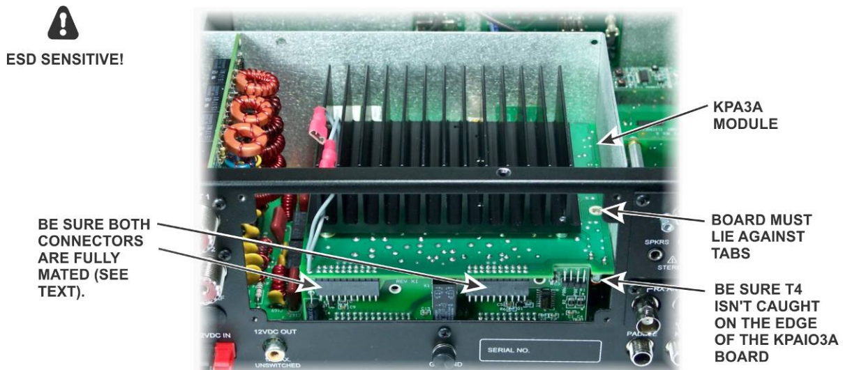
Figure 15. Mounting the KPA3A Module.
