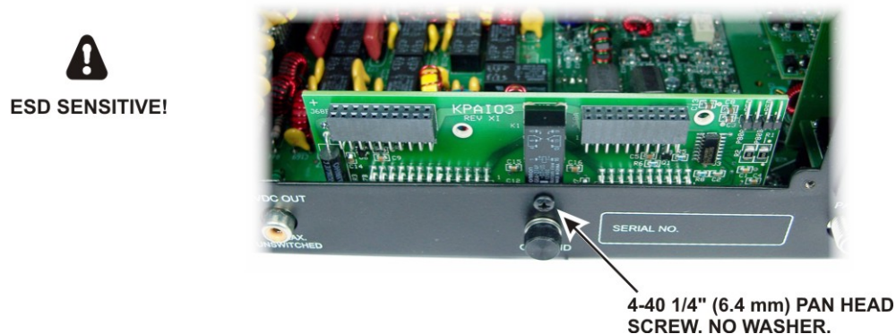
Figure 11. Installing the KPAIO3A Module.
